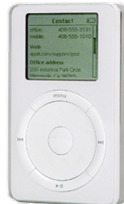
The first generation iPod was simply a hard drive with controls for playing audio files.
